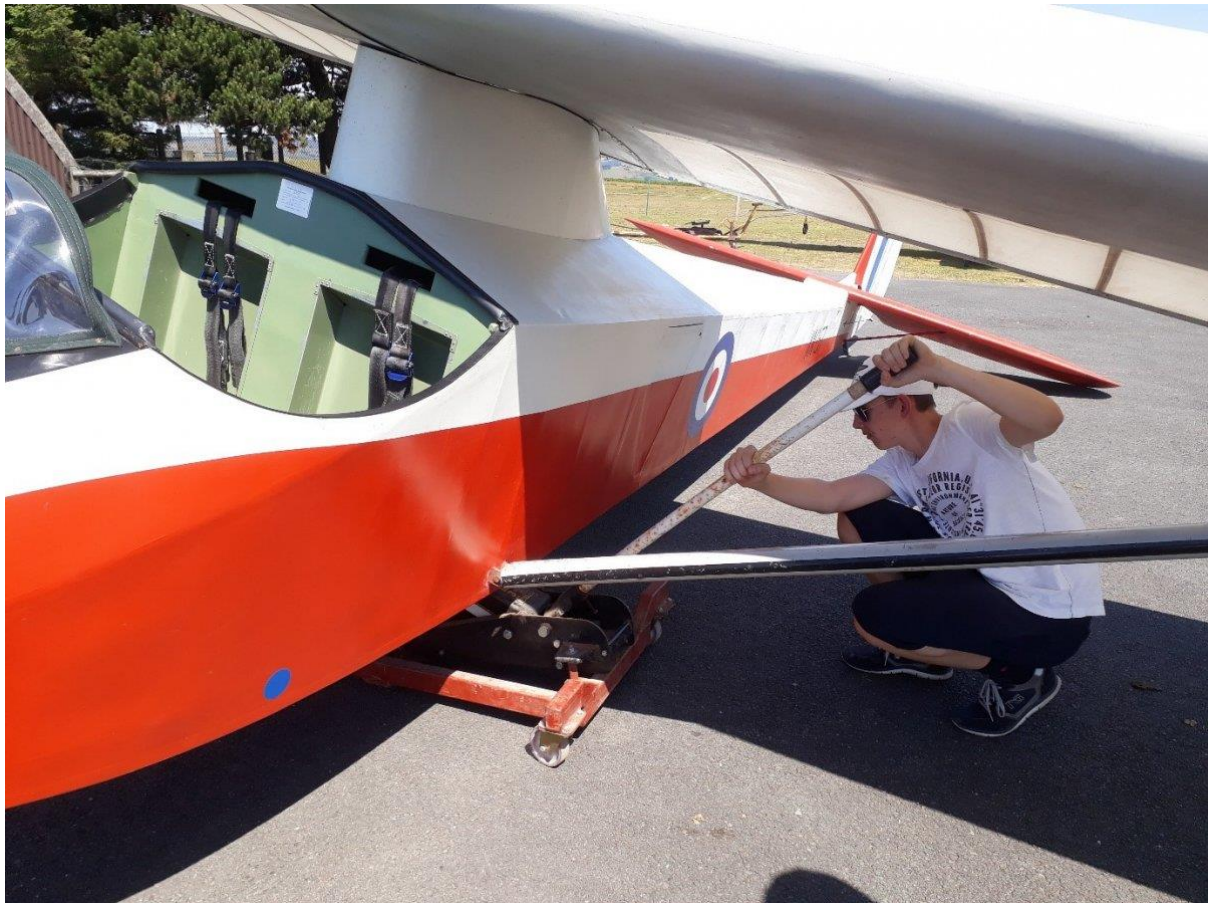
(Above:) Ivan jacking up the T21; (Below:) Theo manoeuvring the K8 out of the hangar
